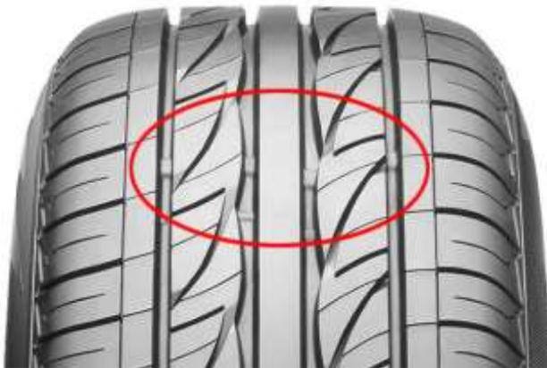
Show Me Tell Me answer 14 explains there should be a minimum of 1.6mm of tyre tread depth to remain safe and legal whilst driving. The picture above shows the tread depth has not yet reached the tyre wear indicators. Keep a check on the tyre wear indicators. If the tyre tread depth gets close to these indicators, it's time for a tyre change.
